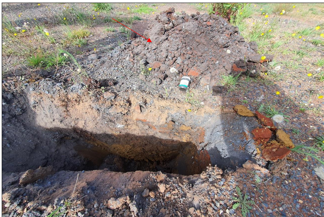
Photo.6. Representative photo of the fill material observed at AEC2.
